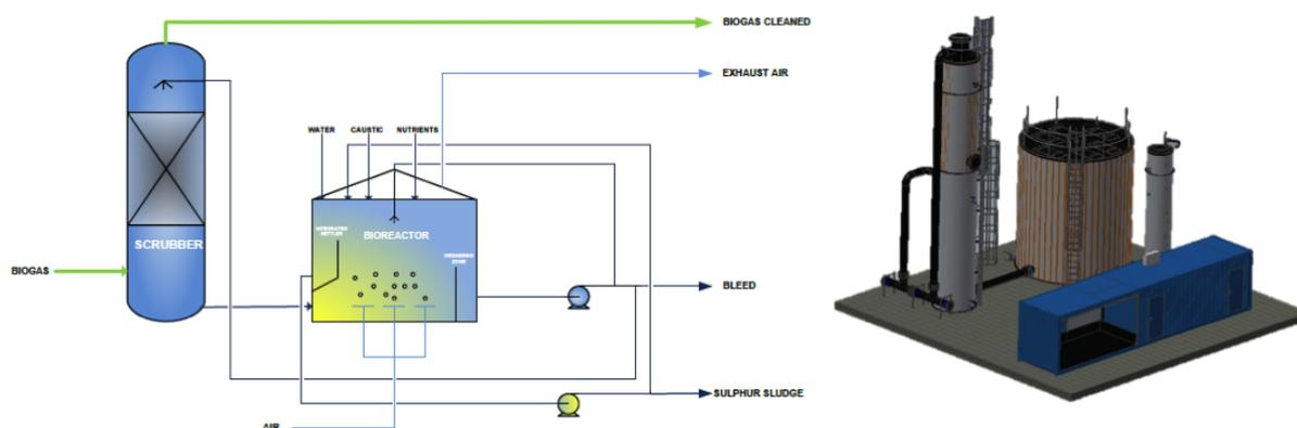
Figure 3. Schematic process of Sulfurex® BR with an integrated settler (left). 3-D drawing of a Sulfurex® BR (right).
