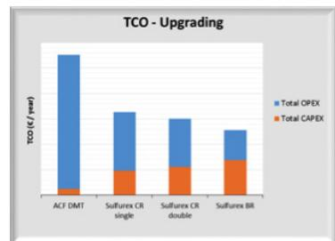
Figure 4. Business case analysis for a general case (Flow 350 Nm<sup>3</sup>/h, 55% of CH<sub>4</sub>, 44% of CO<sub>2</sub> and 4000 ppm of H<sub>2</sub>S). Above Desulfurization selection sweet spot selection. Below, Total Cost of Ownerships for three different cases.
